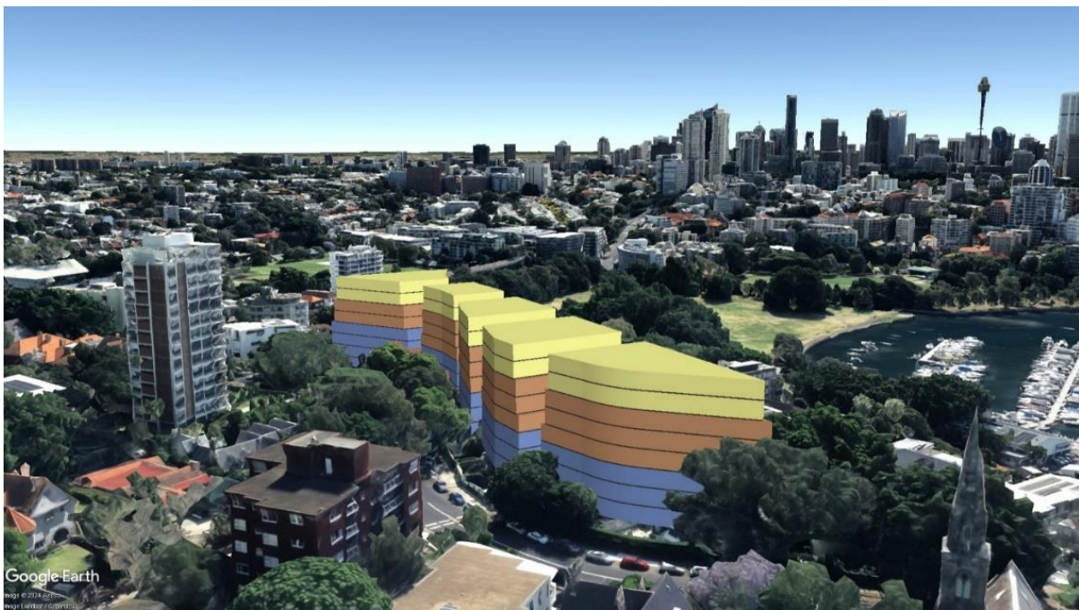
Figure 1: View south-west to Darling Point Road, Darling Point with indicative building envelopes under existing controls (blue), reforms (orange) and reforms plus Housing SEPP AH bonus (yellow).
